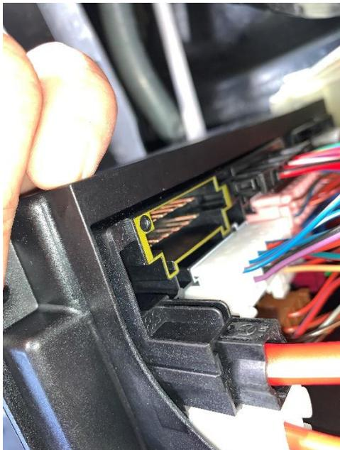
To access the underside of the SAM there are 4 screws one in each corner, please note there are plastic turrets around the screws, I removed these to get access to the torx screw then realised they are there to STOP screws falling into the SAM, please DO NOT remove these turrets and use long reach Torx bits.
