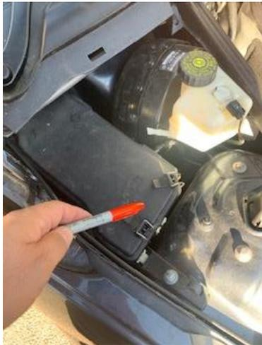
You need to connect this wire to connector 21 pin 8 this is the yellow connector underneath the SAM. It will then be fused by fuse f13 7.5a
