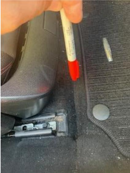
Neatly pack the wires into the floor with the main wiring and close the covers you will now be left with a red/black wire, feed this through to the front SAM.
