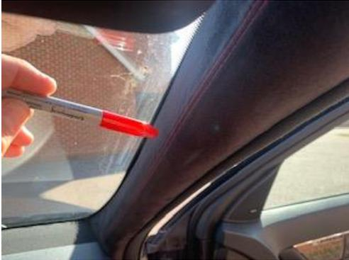
Feed the wiring behind the dash following the existing wiring and pull it down into the drivers footwell, cable tie the new wiring to the existing loom in the window pillar, be very careful of the curtain airbag.
